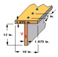
Two wooden planks with the dimensions shown are fastened with nails and subjected to a vertical shear force as indicated. The maximum force supported by each nail is 80 lb. Determine the maximum applied shear force.
