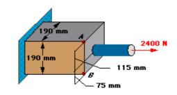
A 2400-N load is applied to a rod, which is fastened to a block as shown. Determine the normal stress at points  ${\cal A}$  and  ${\cal B}$ .
