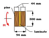
In order to increase the load carrying capability of a pine joist ( $\emph{E}$ = 11 GPa), a 6-mm-wide laminate ( $\emph{E}$ = 35 GPa) is placed between two 44-mm  $\times$  300-mm pine timbers. The pine timbers can sustain a maximum normal stress of 17 MPa. Determine the difference between the maximum moment that can be supported by a 94-mm  $\times$  300-mm pine beam and the beam section shown (with the laminate).
