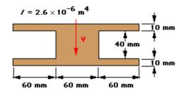
The beam section shown is made from a material that can withstand a maximum shear stress of 55 MPa. Determine the maximum transverse shear force that can be applied to the section.
