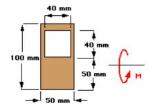
A segment of beam is subjected to pure bending about its horizontal centroidal axis. The cross-section of the beam has the dimensions shown. The allowable tensile and compressive stresses for the beam are 110 MPa and 125 MPa, respectively. Determine the magnitude of the maximum allowable applied moment.
