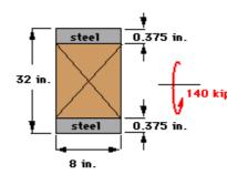
A wooden block is reinforced by steel plates located on the top and bottom surfaces. A 140 kip-ft moment is applied as shown. Determine the tensile stress in the wood and steel reinforcing plates. It is known that
