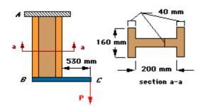
Section  $\mathcal{AB}$  is fixed at  $\mathcal{A}$ , and a load  $\mathbf{P}$  is applied to rigid bar  $\mathcal{BC}$ , as indicated. The allowable tensile and compressive stresses for the material are 180 MPa and 330 MPa, respectively. Find the maximum load  $\mathbf{P}$  that can be applied.
