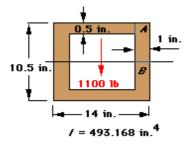
The beam section shown is subjected to the shear force indicated. The top and bottom walls are 0.5-in, thick and the side walls are 1-in, thick. Determine the shear stress at  $\mathcal{A}$  and  $\mathcal{B}$  (the neutral bending axis).
