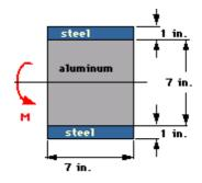
A composite beam is constructed by bonding two steel strips to an aluminum core as shown. The maximum allowable normal stress in the steel is 30 ksi, and in the aluminum it is 18 ksi. Determine the maximum allowable bending moment that can be applied to the beam. Note that
