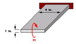
A cantilevered beam is subjected to a bending moment as shown. The normal stress in the beam is 30 ksi. Assume the beam is made from steel, with  $\mathcal{E}=29\times10^6$  psi. Determine the radius of curvature of the beam.
