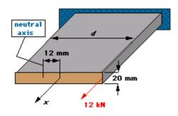
For the cantilevered beam shown, determine the beam width  ${\it d}$  required so that the neutral axis is located 12 mm to the left of the centroid of the beam.
