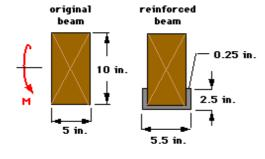
In order to increase the load carrying capability of a wooden beam, a 10.5-in.  $\times$  0.25-in. reinforcing strap is bent into the shape of a bracket and placed on the bottom of the beam. A bending moment of 175 kip-in. is applied as shown to each beam. Determine the ratio of the maximum tensile stress in the wood for both beams,  $\sigma_{\text{orig.}}/\sigma_{\text{reinforced}}$ . The wood and reinforcement have elastic moduli of  $\mathcal{E}_{\text{rein.}} = 30 \times 10^6$  psi.
