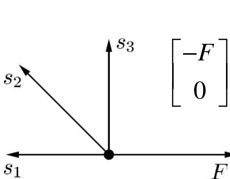
$$\begin{bmatrix} -F \\ 0 \end{bmatrix} = \begin{bmatrix} -1 & -\frac{\sqrt{2}}{2} & 0 \\ 0 & \frac{2}{\sqrt{2}} & 1 \\ 0 & \frac{\sqrt{2}}{2} & 1 \end{bmatrix} \begin{bmatrix} S_1 \\ S_2 \\ S_3 \end{bmatrix} = -[\mathbf{d}_1 \quad \mathbf{d}_2 \quad \mathbf{d}_3] \cdot \mathbf{S} \rightarrow -\mathbf{F} = -\mathbf{B} \cdot \mathbf{S} \rightarrow \mathbf{F} = \mathbf{B} \cdot \mathbf{S}$$
